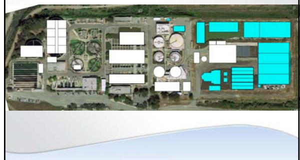
Full Site Layout – MBR Activated Sludge
