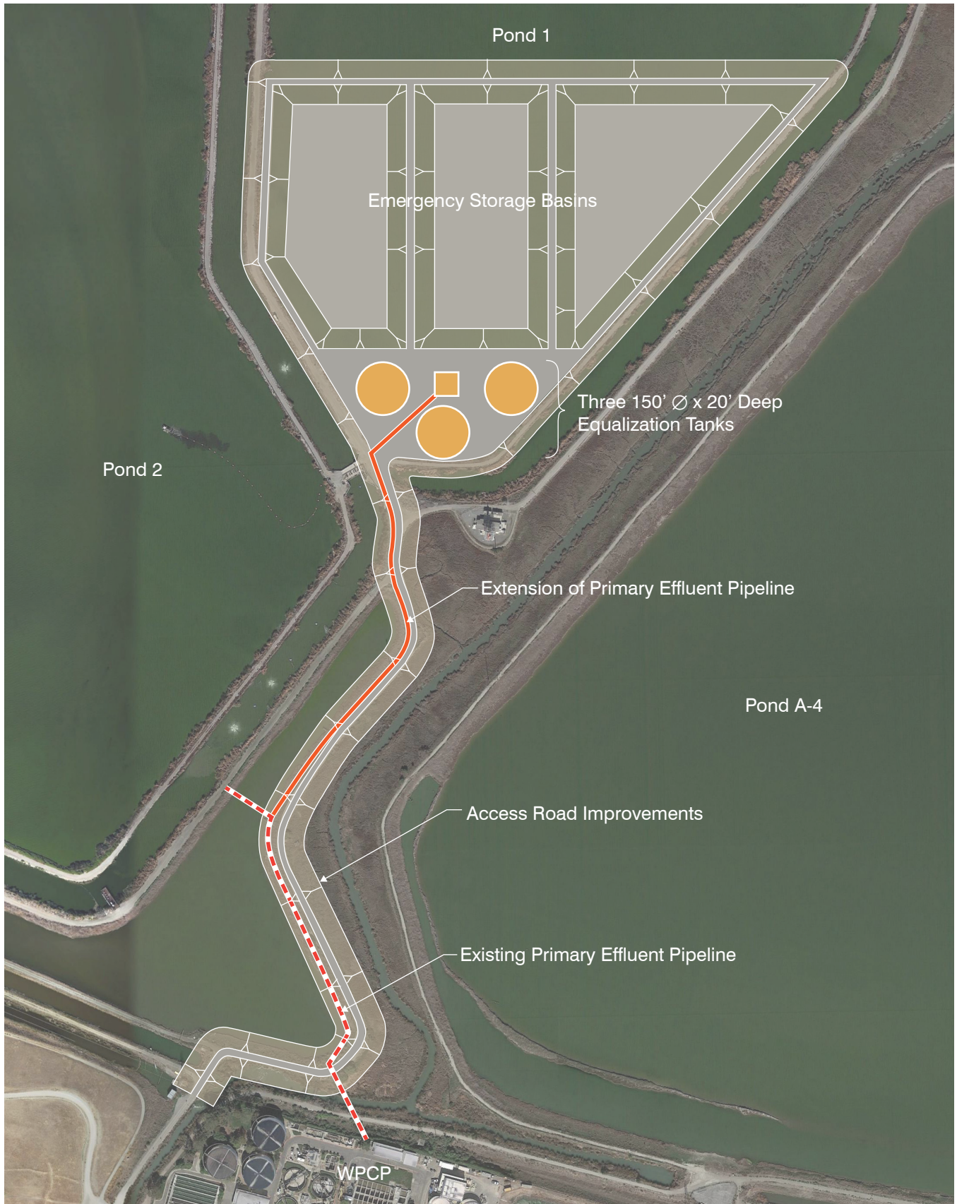
Figure 9 PROPOSED EQUALIZATION LOCATION SECONDARY TREATMENT MASTER PLAN AND PRIMARY TREATMENT DESIGN CITY OF SUNNYVALE
