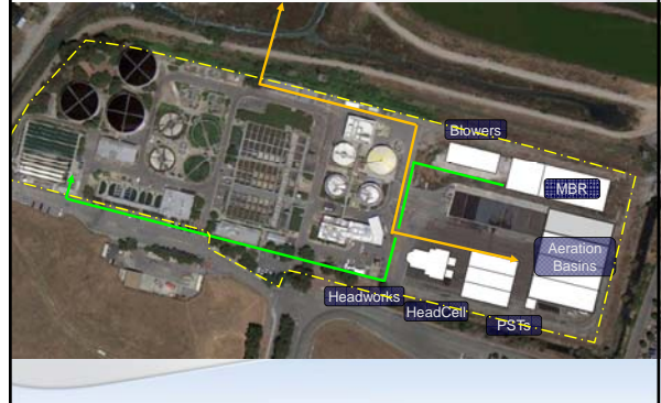
Site Layout – MBR Activated Sludge
