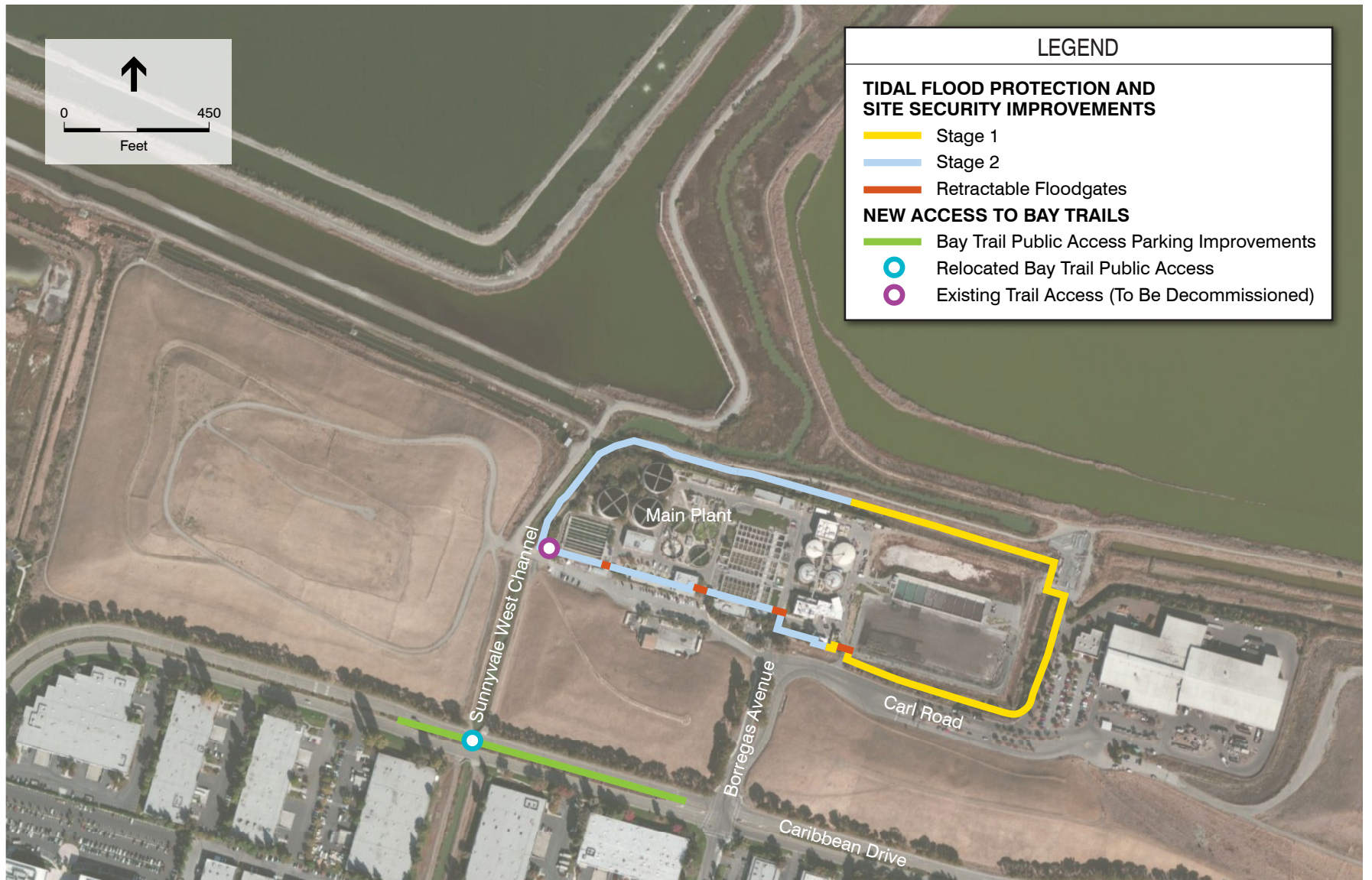
Figure D.4 SITE PERIMETER AND OTHER CIP IMPROVEMENTS CIP IMPLEMENTATION (MBR) MASTER PLAN AND PRIMARY TREATMENT DESIGN CITY OF SUNNYVALE
