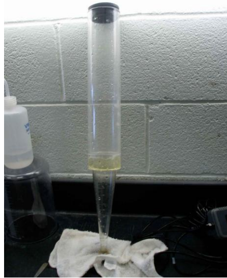
Figure 5. Modified Imhoff Cone for SES Measurements
