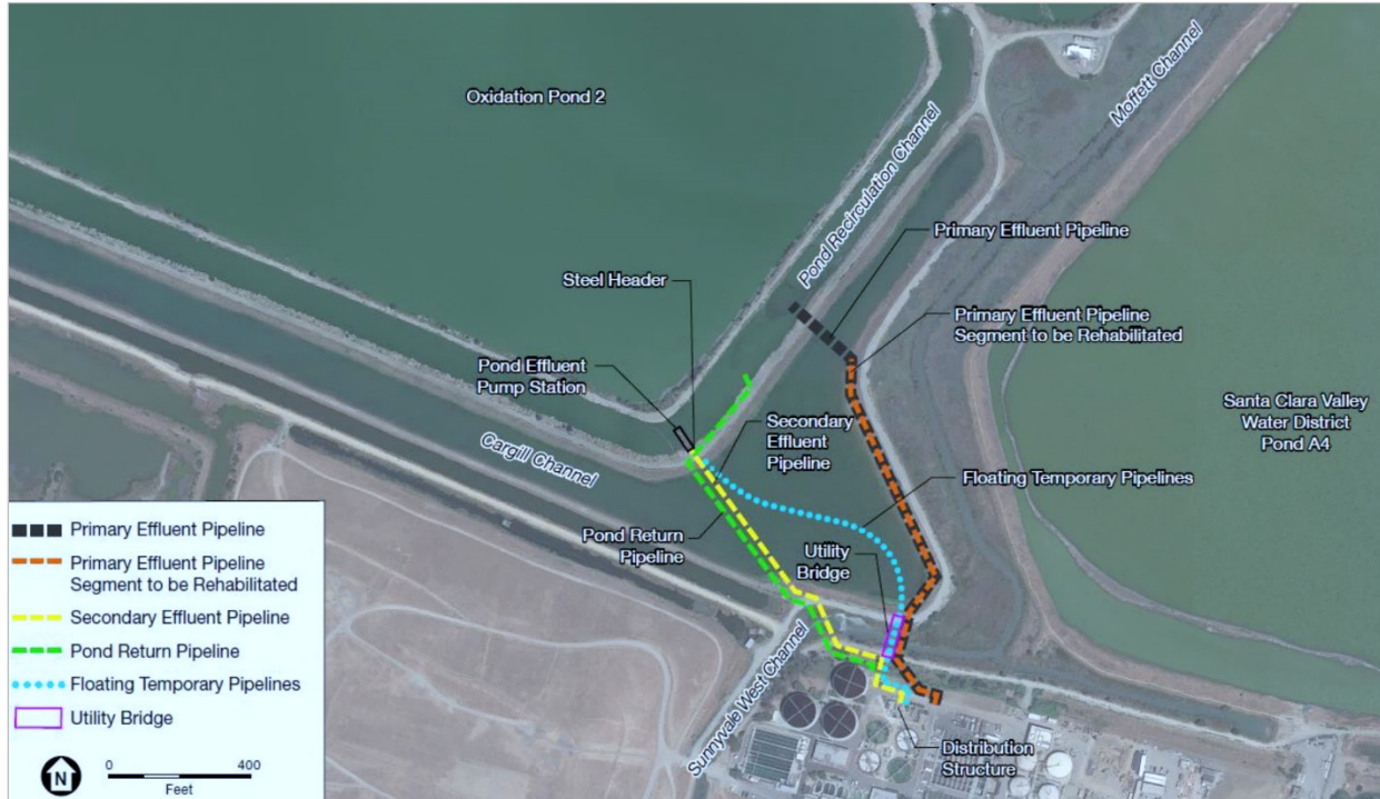
Figure 30: Pipeline Replacement Project configurations and alignments
