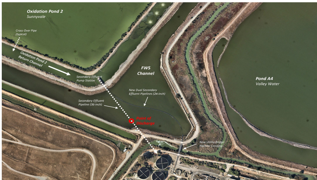
Figure 29: Alignment of WPCP process piping and point of unauthorized discharge in FWS Channel
