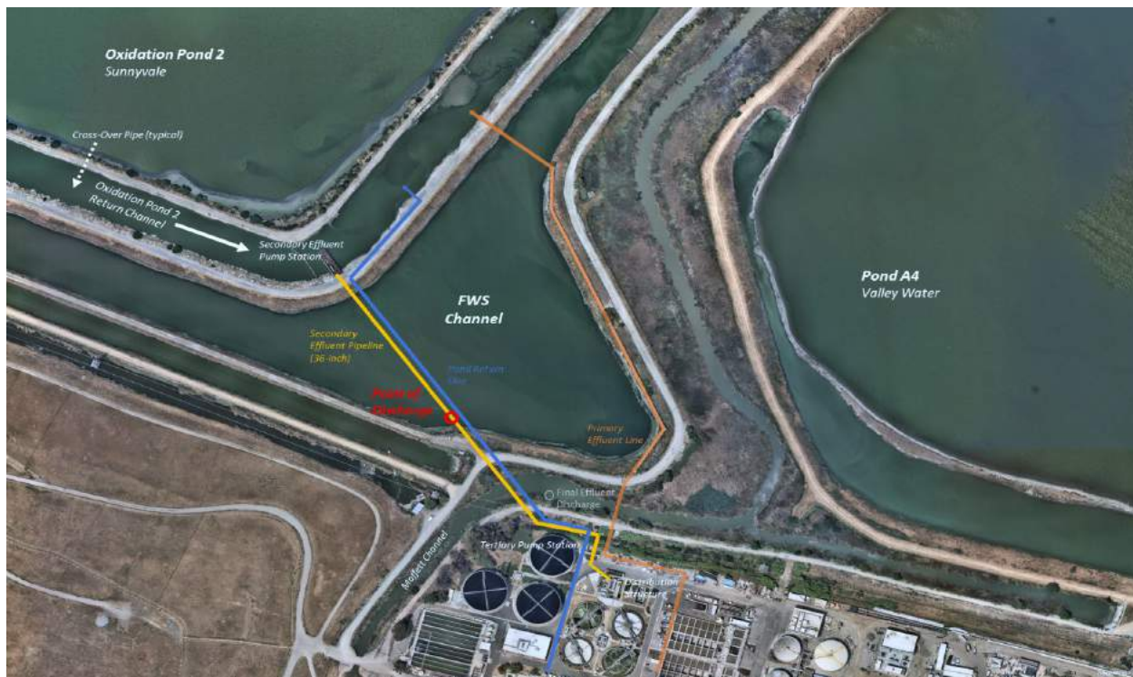
Figure 29: Alignment of WPCP process piping and point of unauthorized discharge in FWS Channel
