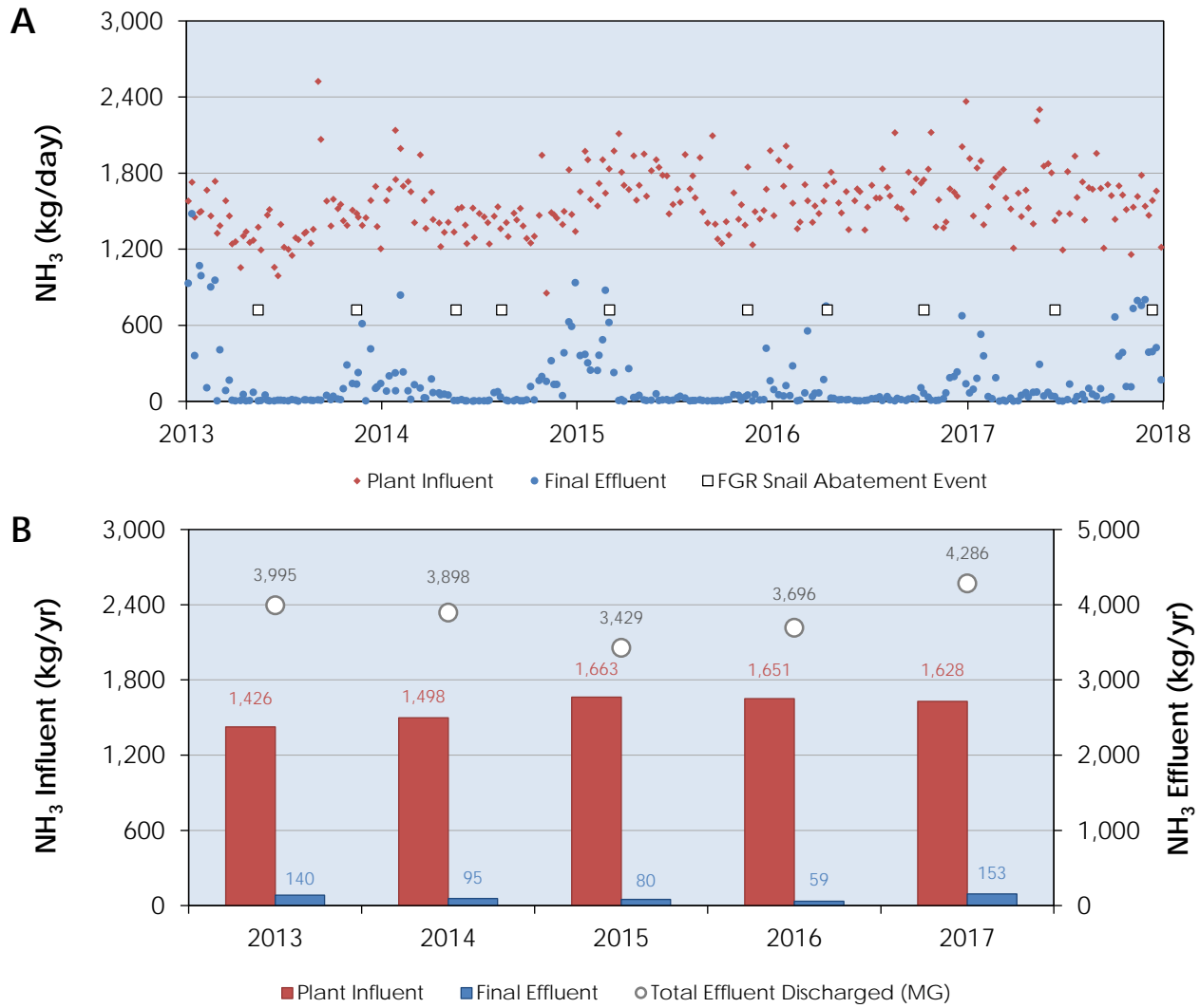
Figure 21: Average A) Daily and B) Annual Ammonia Loading Rates and Total Effluent Discharged from 2013-2017
