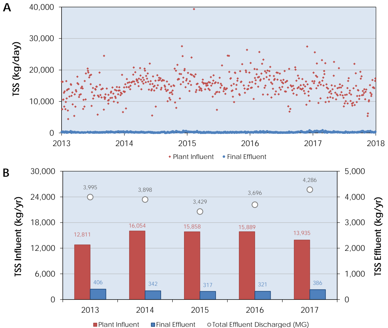
Figure 19: Average A) Daily and B) Annual TSS Loading Rates and Total Effluent Discharged from 2013-2017
