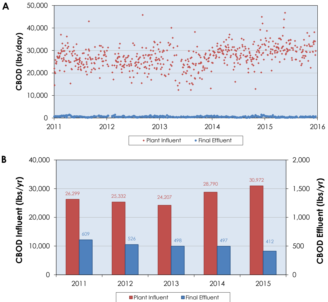
Figure 21: Average A) Daily and B) Annual CBOD Loading Rates at the WPCP from 2011-2015
