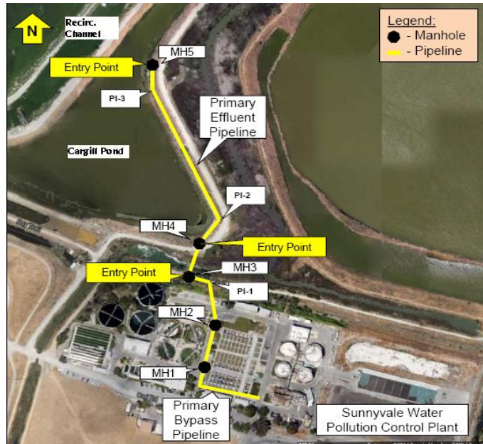
Figure 34: Primary bypass pipeline and Primary effluent pipeline inspection
