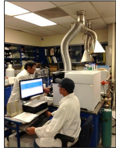
Figure 10: Laboratory Technician Analyzing Wastewater Effluent Sample on the WPCPs new ICPMS
